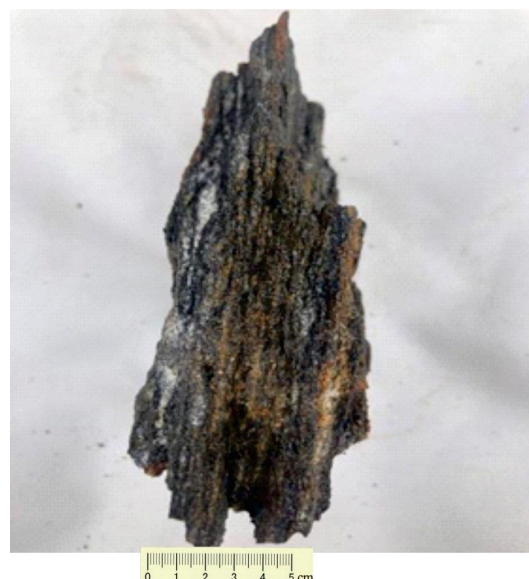
Fig.3 Flake structure of graphite ore
