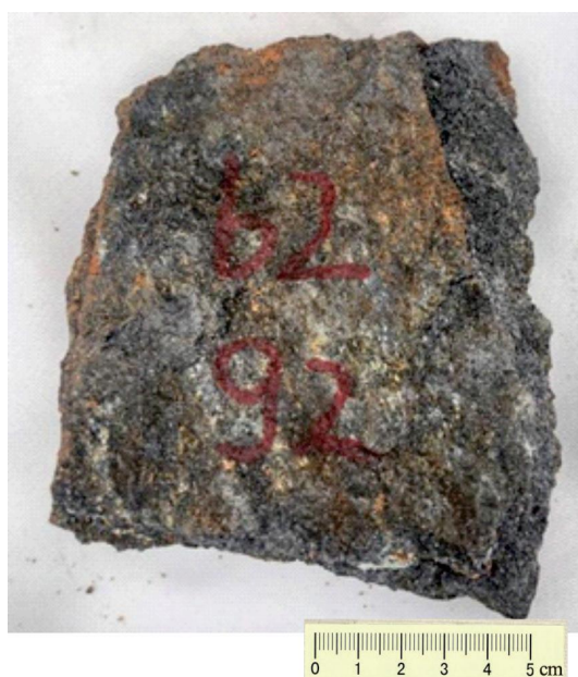
Fig.2 Graphite aligned along the foliation plane
